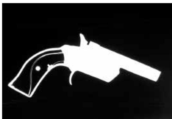
Figure 10. Ultrasound of a piece of evidence, packaged in a cardboard box and labeled as a homemade weapon .To avoid the dangers of manipulation a ultrasound is taken before opening the box to check if the trigger is in its default position, minimizing the risk of accidentally shooting it.
