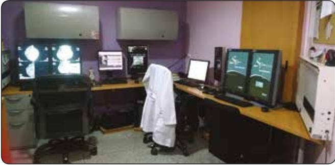
Figure 3. High resolution monitors (5 and 5.5 Megapixels). Screens for mammograms, BARCO®.
