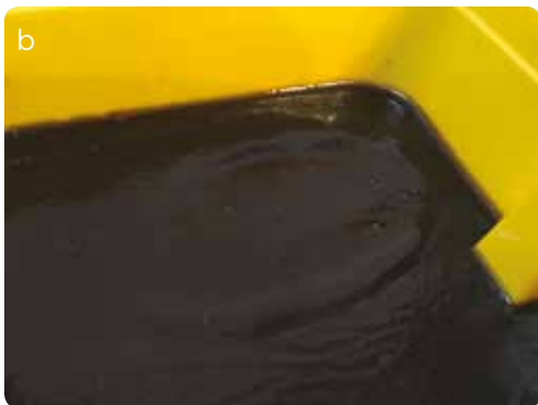
Figure 6. a) Repair process of coarse rupture using high temperature hair dryer. b) Appearance with finished repair.
