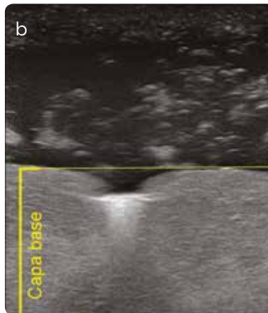
Figure 2. a) Base layer with few bubbles. b) Ultrasound image of the base layer.
